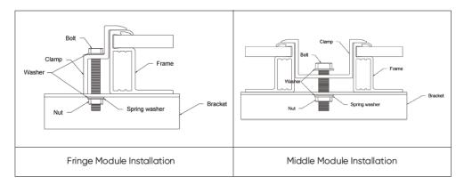
Under no circumstances should the clamps touch the glass or deform the frame of the module. The front contact surface between the clamp and the frame must be smooth, otherwise the frame may be damaged and result in the damage of the module.
